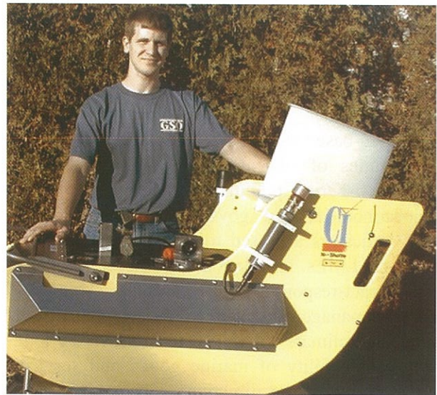
Figure 5. Northeast Fisheries Science Center Systematic measurements are made of LMEs by using towed bodies such as the Mariner Shuttle, depicted here. The electronically produced outputs from Mariner Shuttle sensors show vertical profiles of depth, temperature, salinity, chlorophyll, oxygen, and sigma T (density) based on undulating continuous sampling [12].
